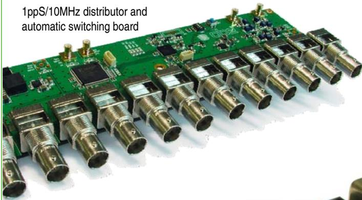
1ppS/10MHz distributor and automatic switching board
